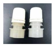
Fig.3) Spouts and caps. 100% recycled material (left) and 100% new material (right)
